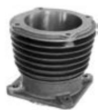
Made from nodular cast iron outer side surrounded by channels for better cooling capacity. Separate assembly to body provide easy service and replacement.
