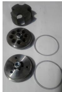
Each compressor have suction and delivery valve system which designed as per compressor capacity
