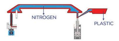
The blank areas inside of the injection mould fill by plastic resin and nitrogen. By this way the compactor pressure disperses well to all sides of injection mould which provide well forming, create less air bubble and finally product surface have smooth finishing.
